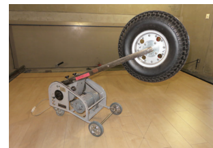
Test for reduction of transmitted impact sound by floor coverings
