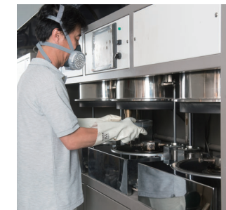
Asphalt extraction test for asphalt mixture
