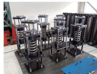
Creep test of post-installed anchor
