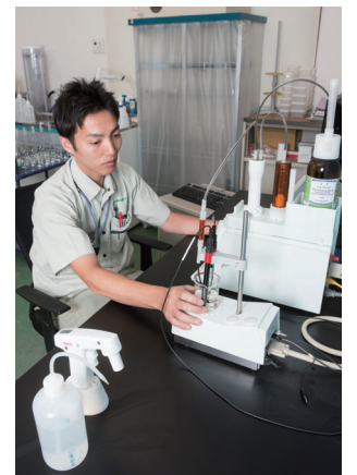
Test for chloride ion content
