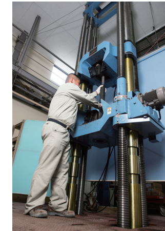
Tensile test for reinforced steel bar by 2000kN universal testing machine
