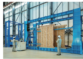
Deformation test of exterior finishing materials
