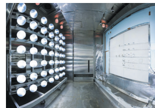
Durability tests of exterior materials of buildings by solar radiation
