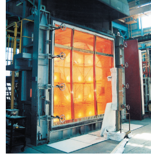
Fire-resistance test of windows and doors
