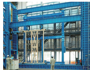
In-plane shear test of bearing wall
