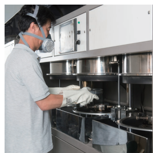
Asphalt extraction test for asphalt mixture
