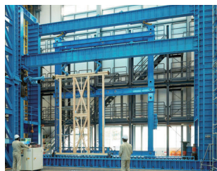
In-plane shear test of bearing wall
