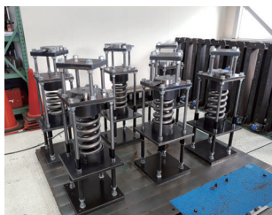
Creep test of post-installed anchor
