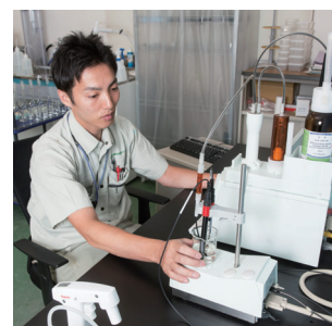
Test for chloride ion content
