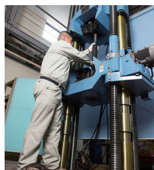
Tensile test for reinforced steel bar by 2000kN universal testing machine
