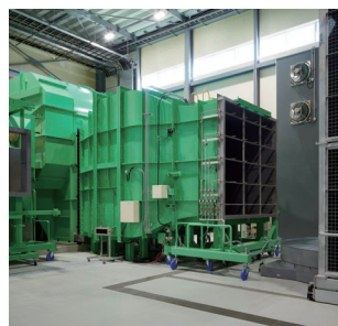
Watertight and wind pressure resistance test using real wind
