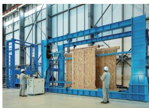
Deformation test of exterior finishing materials
